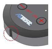
Insert the control unit aligning it with the shorter marking on the holder at position (1) and turn it clockwise until it aligns with the longer marking on the holder at position (2):
